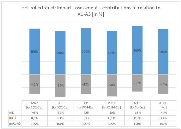
The figure above shows the relative contribution of the production stages (Module A1-A3), waste treatment (Module C3) and the benefits and loads beyond the product system boundary (Module D).
